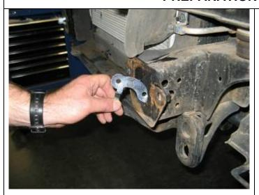
27. Insert a nut plate into the chassis hole as shown
