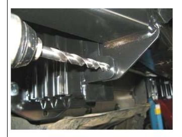
63. Using an electric drill and a 10.0 mm drill bit, drill two pinning bolt holes through the bull bar upright each side using the holes in the mount bracket flanges as a guide. One hole is located in the lower lug of the mount face and one up above the welded nuts. Use access through the light surround opening for the top hole.
