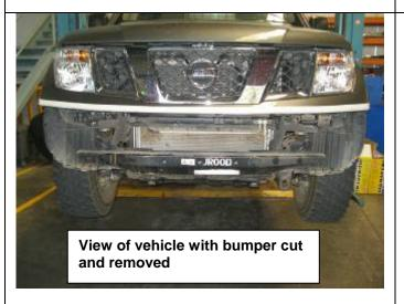
16. Clean up the cut edges of the bumper bar with a file or fine sand paper.
