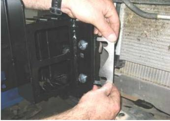
36. Insert packing plates as shown, these mate around the shape of the chassis end plate and are sandwiched in between the back face of the mount bracket (impact absorber) and the front flange of the angle bracket previously installed to the side of the chassis
