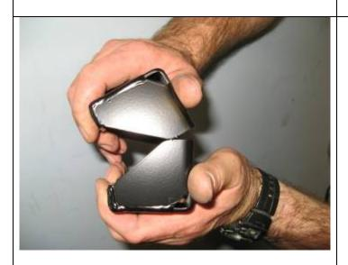
28. Break apart each of the bracket sets as shown. These are handed to fit around the weld nut on the rear of the chassis end plate.
