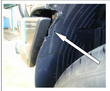
72. With the two horizontal cuts done, cut down from the end of the top cut to the bottom cut vertically (the inner guard needs to have clearance to the bull bar wing return as shown).
