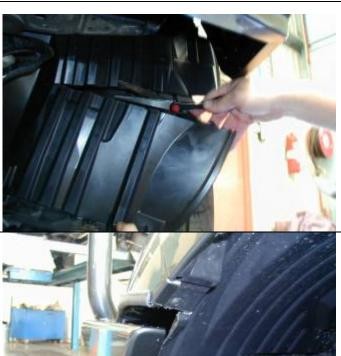
73. With part of the inner guard now trimmed to clear the wing return the remaining part of the inner liner that hangs down below the bottom of the wing can be trimmed off horizontally.
