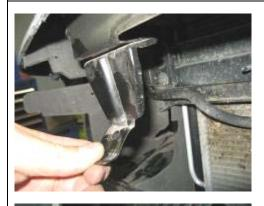
17. Bend up the three metal bumper support tabs to horizontal or alternatively cut them off
