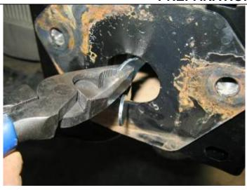
33. Bend back tabs on nut plates back into chassis ends with pliers as shown
