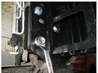
59. Now the bull bar is in position, all of the bolts on the chassis mount can be tightened firmly to specified torque.
