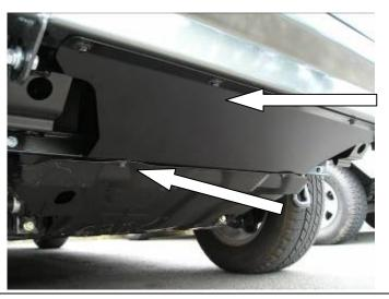
67. Attach the stone tray to the under side of the bull bar with the black M6 bolts, flat washers & spring washers.
