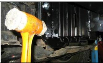
56. If the bull bar is not central to the vehicle, tap the outer corners of the mount bracket flanges as shown.
