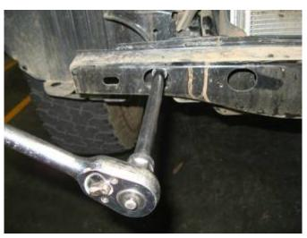
25. The four bolts that hold the bumper reinforcement beam can now be removed and set aside.
