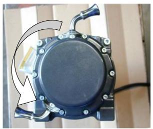
43. Remove the cap head screws retaining the gearbox to the winch drum. Carefully lift the gearbox a small amount (5 mm) and rotate144 degrees counter clockwise (four hole spacings) and re-fit the cap screws. This places the winch handle in the correct orientation.
