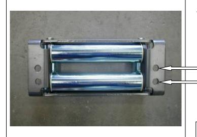
46. Using a 12mm drill bit, mark & drill two new holes in the roller fairlead 25mm below the original holes.
