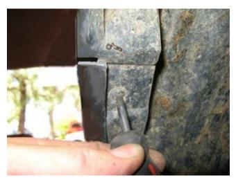
6. Remove the screws securing the fender liners to bumper in the forward wheel arch areas
