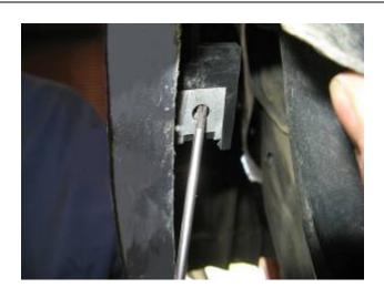
7. Remove the speed nut from the bumper on each side
