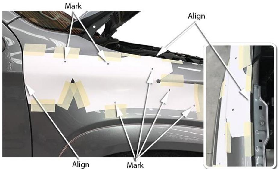
Drill a pilot hole for each of the marked hole positions.
