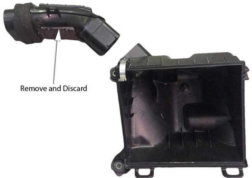
Measure and mark two hole positions on the air cleaner base inlet approximately 10mm in from the end of the air cleaner base inlet and 23mm (long side) and 15mm (short side) down from the radius of the inlet as shown.
