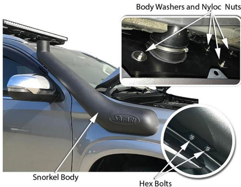
Align the air entry hose (item 12) for best fitment (*Ensure the air entry hose is installed hard up against the shoulder of the snorkel body outlet*), correctly position the hose clamps at either end of the air entry hose and tighten.
