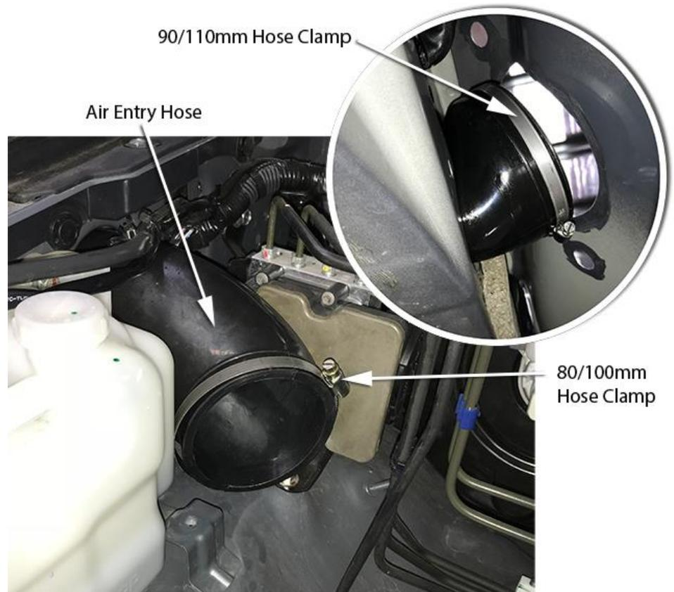
Re-install the air cleaner base, guiding the air cleaner inlet adaptor into the air entry hose, fasten the air cleaner housing using standard mounting bolts.
