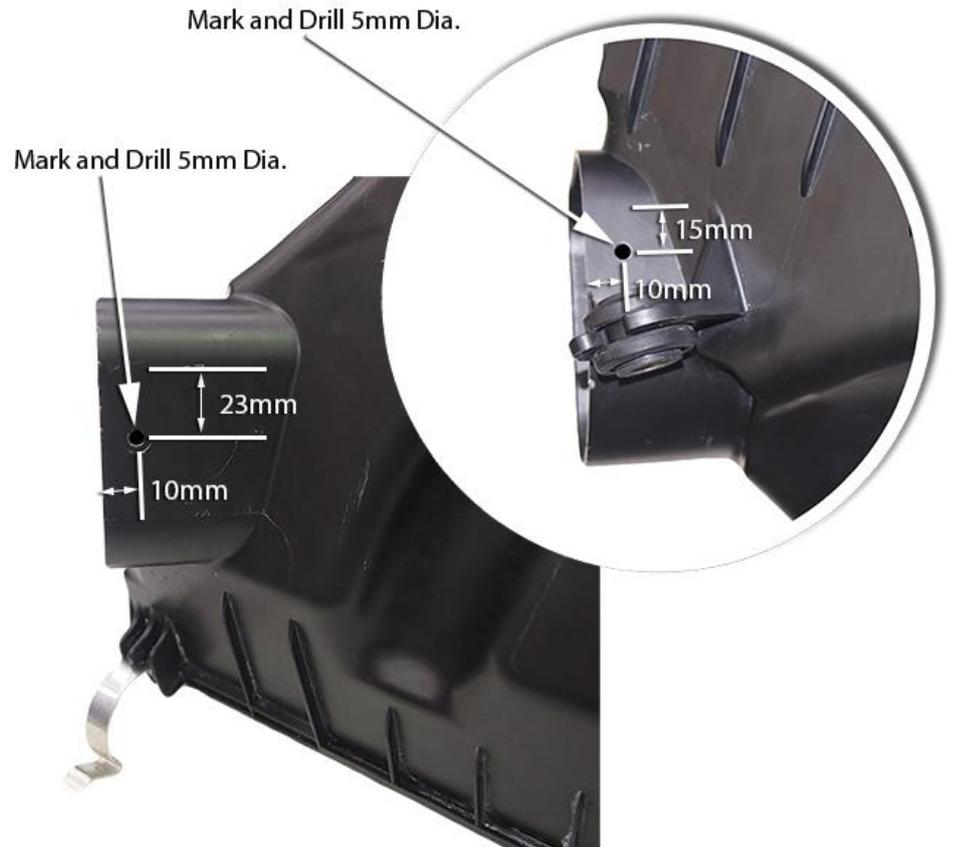
Install the air cleaner inlet adaptor (item 10) into the air cleaner base inlet, drill the two 5.0mm holes through the air cleaner base and into the air cleaner inlet adaptor.
