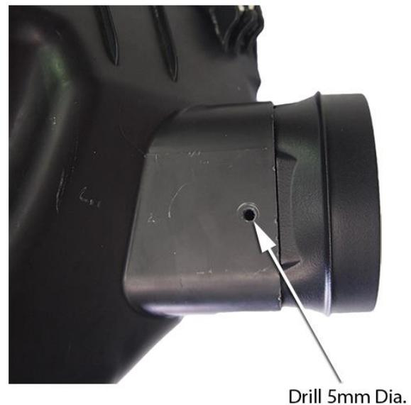
Apply adhesive sealant to the inside of the air cleaner base inlet and the outside of the air cleaner inlet adaptor (item 10).
