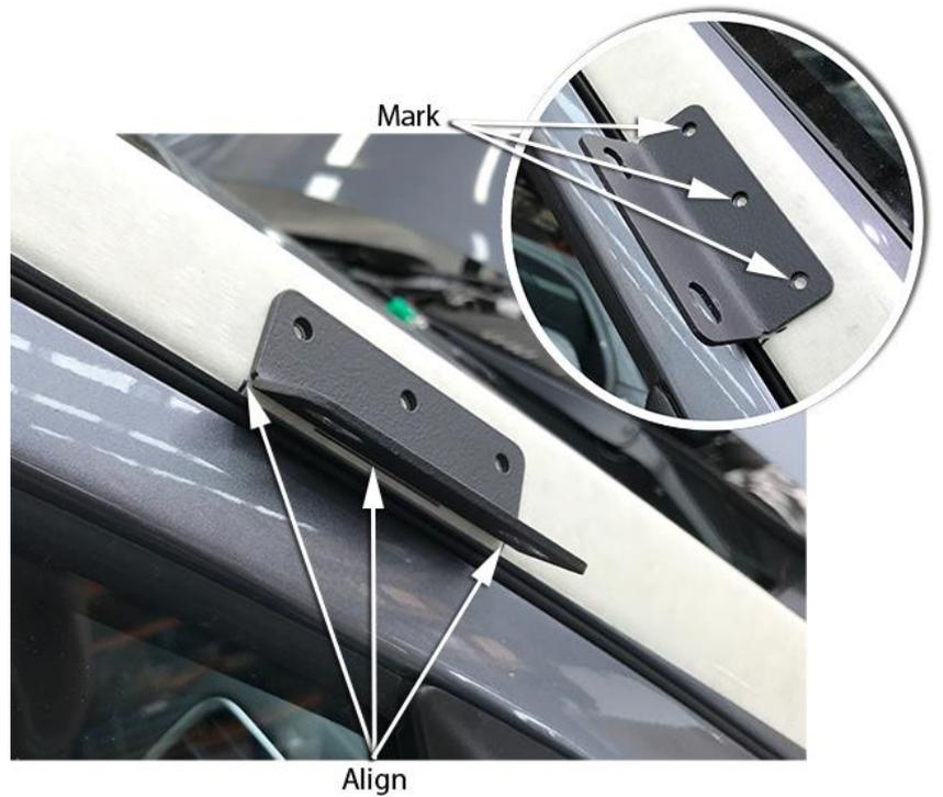
Drill a pilot hole at each of the three marked positions, drilling through both the A-pillar panel and inner panel.
